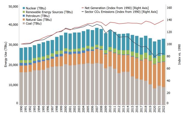
Figure 3-9: Fuels Used in Electric Power Generation and Total Electric Power Sector CO<sub>2</sub> Emissions
