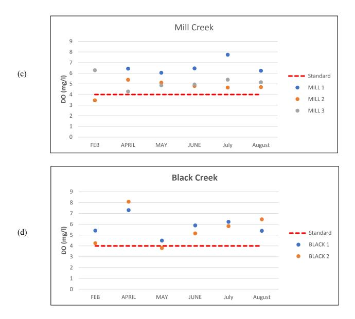
Figure 3.3: Dissolved Oxygen concentration in (a) Iric Branch, (b) Ash Branch, (c) Mill Creek, and (d) Black Creek
