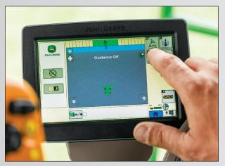
Just like the controls in our combines, GreenStar™3 CommandCenter display puts vital machine information within reach, making it easy for you to make quick guidance or machine adjustments. Plus, you can easily get diagnostic information and monitor machine productivity.
