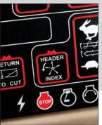
The header index adjusts the reel speed to the ground speed, letting you focus on the platform position instead of adjusting the reel speed as the windrower speed changes due to field conditions. The index maintains a preselected speed based on the ground speed plus an easily adjusted index number. This ensures that when you set the index, the reel will turn fast enough to ensure proper crop flow.
