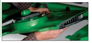
The John Deere cutterbar features individual modules with a diagonal design. Each module slips in and out individually. Just remove seven bolts. The other modules remain attached to the cutterbar frame when the single unit is removed. The cutterbar also can stay on the machine during module removal. The diagonal-cut profile makes alignment easy; reattach the bolts and you're done.
