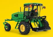
**Transport mode in seconds.** The W100 Series Windrowers transport engine forward with transport speeds up to 27-mph\* (43-km/h) with the W170. High travel speeds are possible due to the increased stability of having the drive wheels push the caster wheels.
