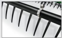
Here's another time saver – quickchange reel teeth. If one breaks, it can be removed and replaced with minimal tools. And it's back to work fast.
