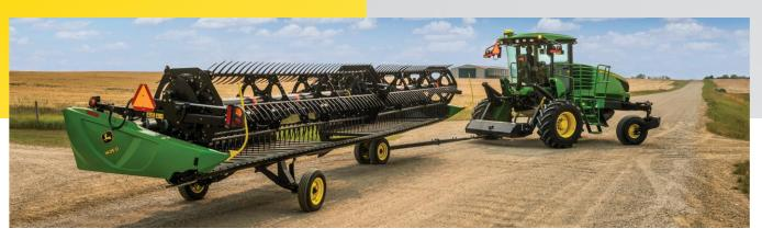
The 430D, 435D, 440D, 1430D, 1435D, 1440D and 1445D Draper models can be equipped with an integral, slow-speed transport system. One person can easily convert the draper from field to transport in minutes without the use of tools. Dual front-dolly wheel tires and two gauge-wheel tires carry the complete weight of the draper when in transport.
