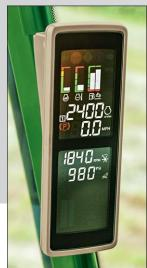
The easy-to-read Primary Display Unit (PDU) makes it easy to monitor machine functions as you run. The full-color display on the right-hand cornerpost shows essential machine information, like fuel level, engine temperature and platform or reel speed. In addition, error messages and warning lights alert you to anything out of the ordinary.
