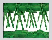
Adjusted properly, impeller conditioning can significantly reduce drydown time. Evenly spaced V-shaped tines are mounted on a rotating tube. As soon as the hay is cut by the disks, the tines carry it through the machine. The hay rubs against itself and against a specially designed, adjustable conditioning hood. This removes the waxy layer from the stems, allowing moisture to evaporate faster.
